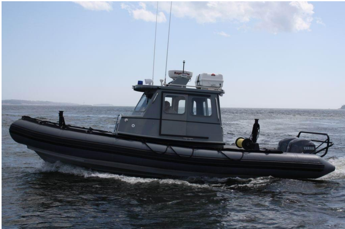
Cabin house made by 4mm marine aluminum.
