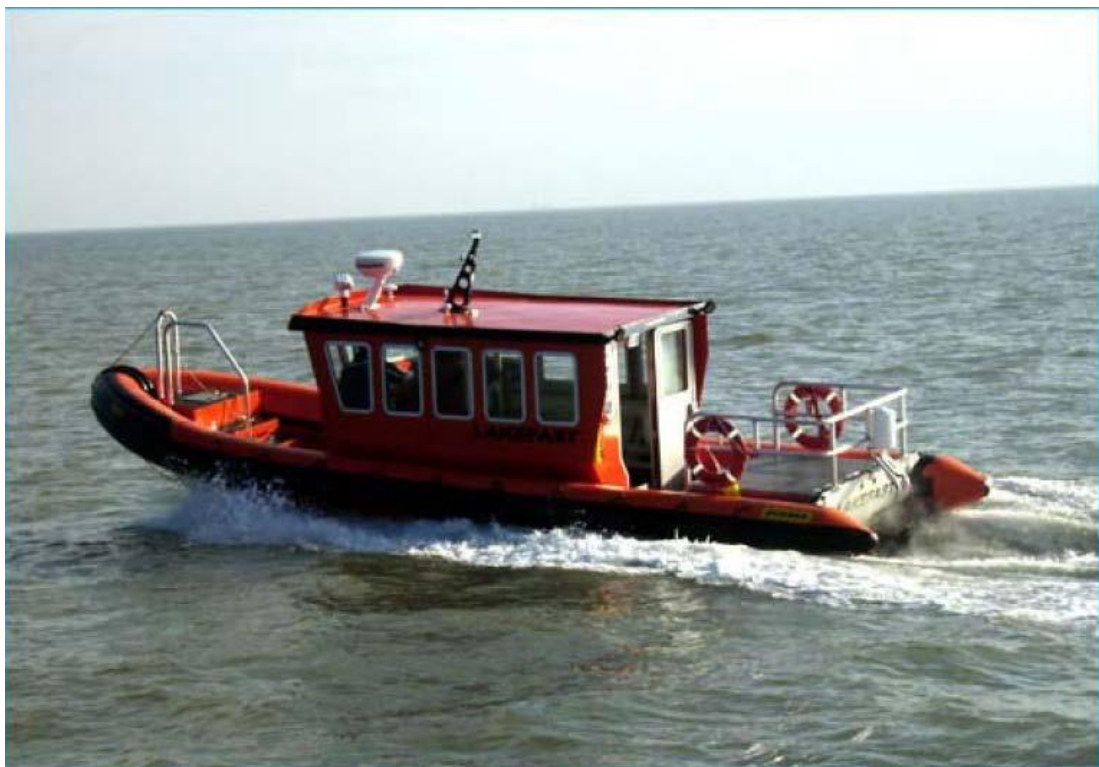
Cabin house made by 4mm marine aluminum.
