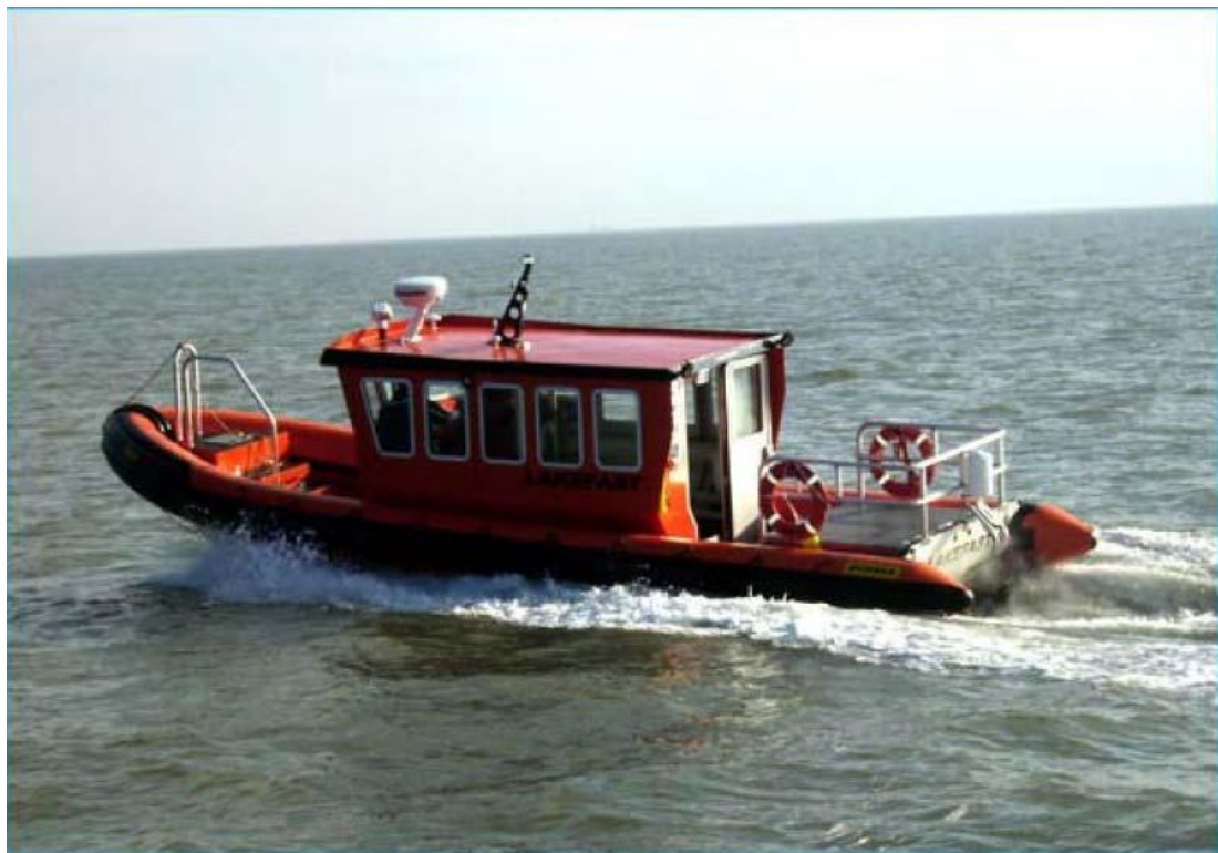
Cabin house made by 4mm marine aluminum.
